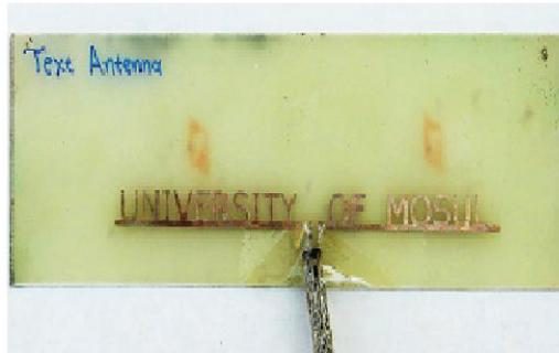
Fig. 11. Photograph of the fabricated Text Antenna.
