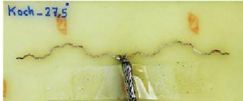
Fig. 17. Photograph of the fabricated K3-27.5 $^\circ$  antenna.
