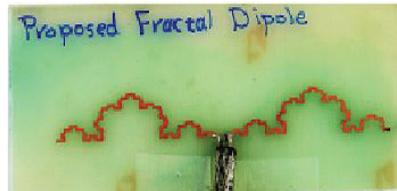
Fig. 18. Photograph of the fabricated (P3) antenna
